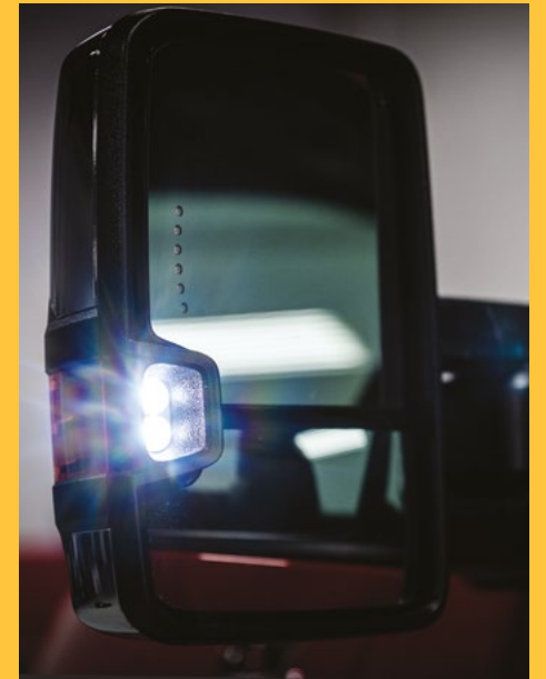
The folding side mirrors can include LED turn indicators plus rear-facing LED lights to illuminate cargo and equipment.
