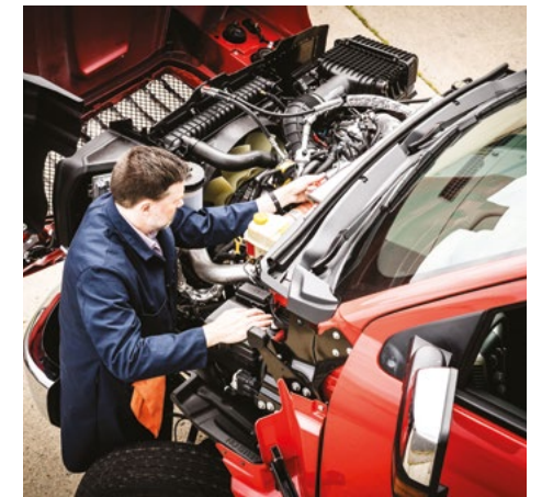
The Forward-tilting hood provides easy access to the engine and routine service points
