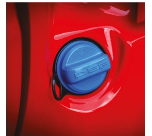
The diesel exhaust fluid (DEF) tank fill point is located near the passenger side door to help avoid mixing the wrong fluids and allows the tank to be filled without opening the hood
